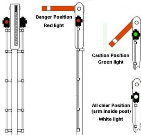
The London & Croydon Railway was one of the first to introduce semaphore signals. These showed three positions by means of an arm mounted in a slotted post. Different indications were given by the position of the arm, horizontal for stop; downwards at 45 degrees for caution; vertical (in fact invisible inside the post) for clear. At night coloured lights were used, red for stop, green for caution, white for clear.
