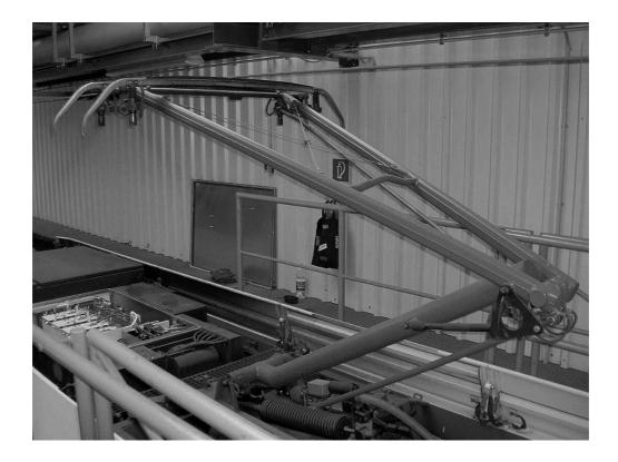
The electric transmission system for modern electric rail systems consists of an upper weight carrying wire (known as a catenary) from which is suspended a contact wire. The pantograph is spring-loaded and pushes a contact shoe up against the contact wire to draw the electricity needed to run the train.
