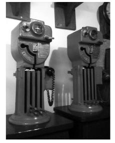
In order to avoid the inevitable delays caused by the signalman having to collect, feed the token through the instrument and then obtain a fresh token various ways have been tried to speed up the process. Interlocking block instruments which could only be used to signal trains in one direction at one time or the use of direction levers in the signalbox which only allowed the signals for one direction to be cleared at any one time.
