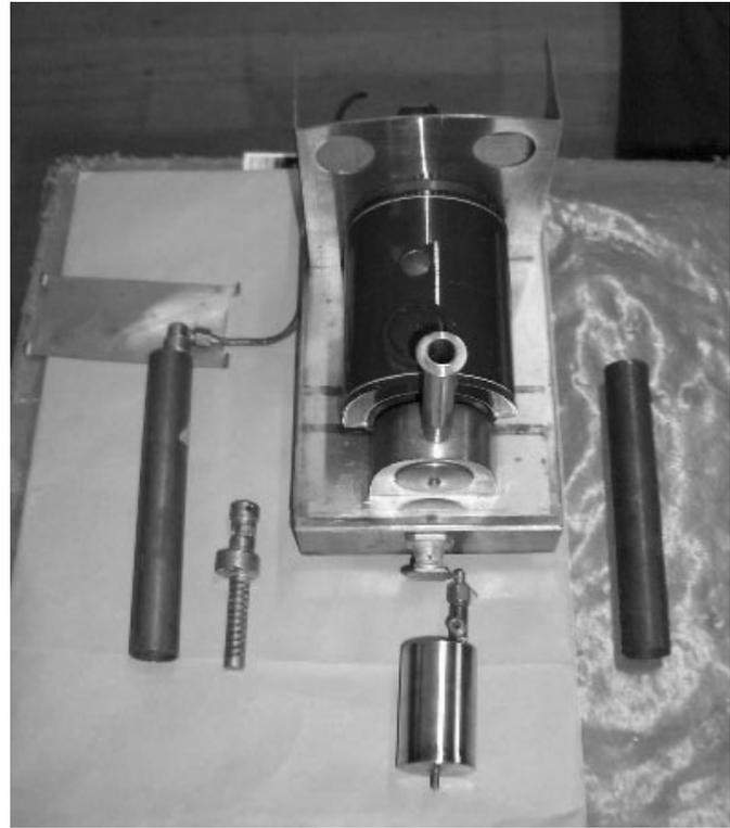
Dave Morris followed with his 16mm Saddle Tank, for his garden railway which he shares with his 3 year old grandson. The loco has a center flue boiler with a butane gas burner – the design of which has caused many problems. The drawings are extremely basic and do not include silly things like dimensions! Reverse is enabled by slip eccentric.
