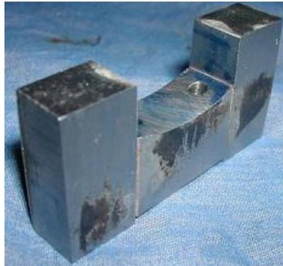
After clamping in position on the web the balance wts were then drilled and the webs tapped M3 for two allen screws. After final shaping they were then screwed on tightly with a everything permanently in since the rebuild and it
